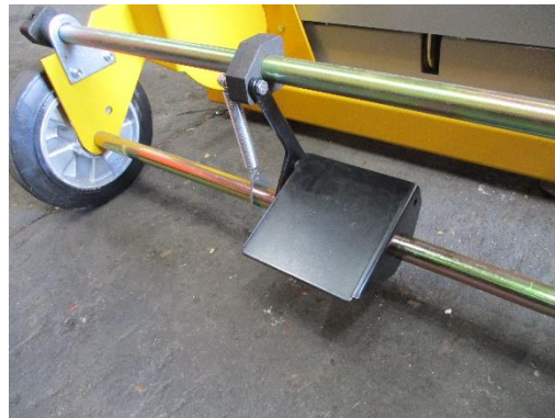
Foot brake (dis-engaged)
